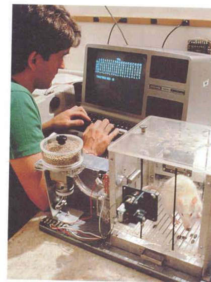
Figure 7.6 Apparatus for Instrumental Conditioning: the Operant Chamber. This photograph shows an operant chamber (often called a 'Skinner box') with a magazine for delivering food pellets. The computer is used to control the experiment and record the rat's responses.
